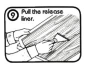
Pull the release liner from the back of the sheet and scrape the veneer to the surface as you pull the liner. Do not use fingers to smooth the veneer. This will result in bubbles. Use the scraper tool. "J" rollers do not result in sufficient nip pressure. Insufficient pressure during application is the major cause of delaminating and checking after application. Pressure sensitive adhesives are very sensitive to lack of pressure. Strive for all possible scraper pressure during application.
